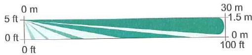
Side View Optional Long Range Coverage (DS970): 30 m x 3 m (100 ft x 10 ft)
